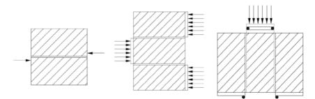
Fig. 2. Test method for shear strength of masonry along the through joint
