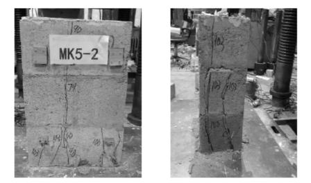
Fig. 4. Failure state of hollow compression standard parts
