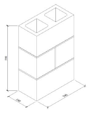
Fig. 1. Sketch map of standard parts (units: mm)
